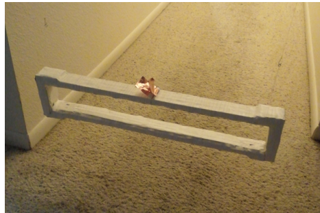
Figure 5.35 Rectangle Suspended with Fishing Lines Note the image presented contains a different number of attached neodymium magnets, but the principle is the same.
